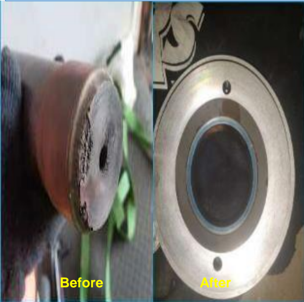
TDBFP R/C valve overhauling and upgradation
